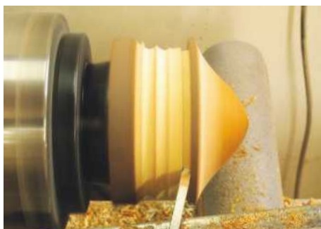
▲ Pic.7 You can see how narrow Les has made the stem; this will give the piece much more definition; do not try and tool the top again at this point as it will be too weak
